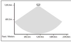
The effective detection area does depend on the height of the ceiling that the alarm unit is mounted on. As a general rule, the effective detection radius when mounted on a ceiling of average height is approximately 9ft/3m.
